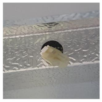
6. Remove connected LED by holding down clip on the underside of the connector. Plug new LED in and reverse steps.
