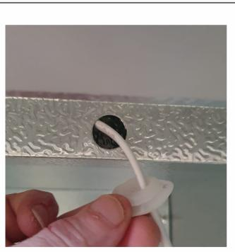
4. Pull out rubber ring from the top right hand side of bottle cooler interior.
